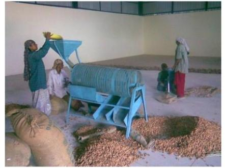
3. Design and modification of groundnut power operated decorticator-M-4A for zone-4 (Hiriyur)
